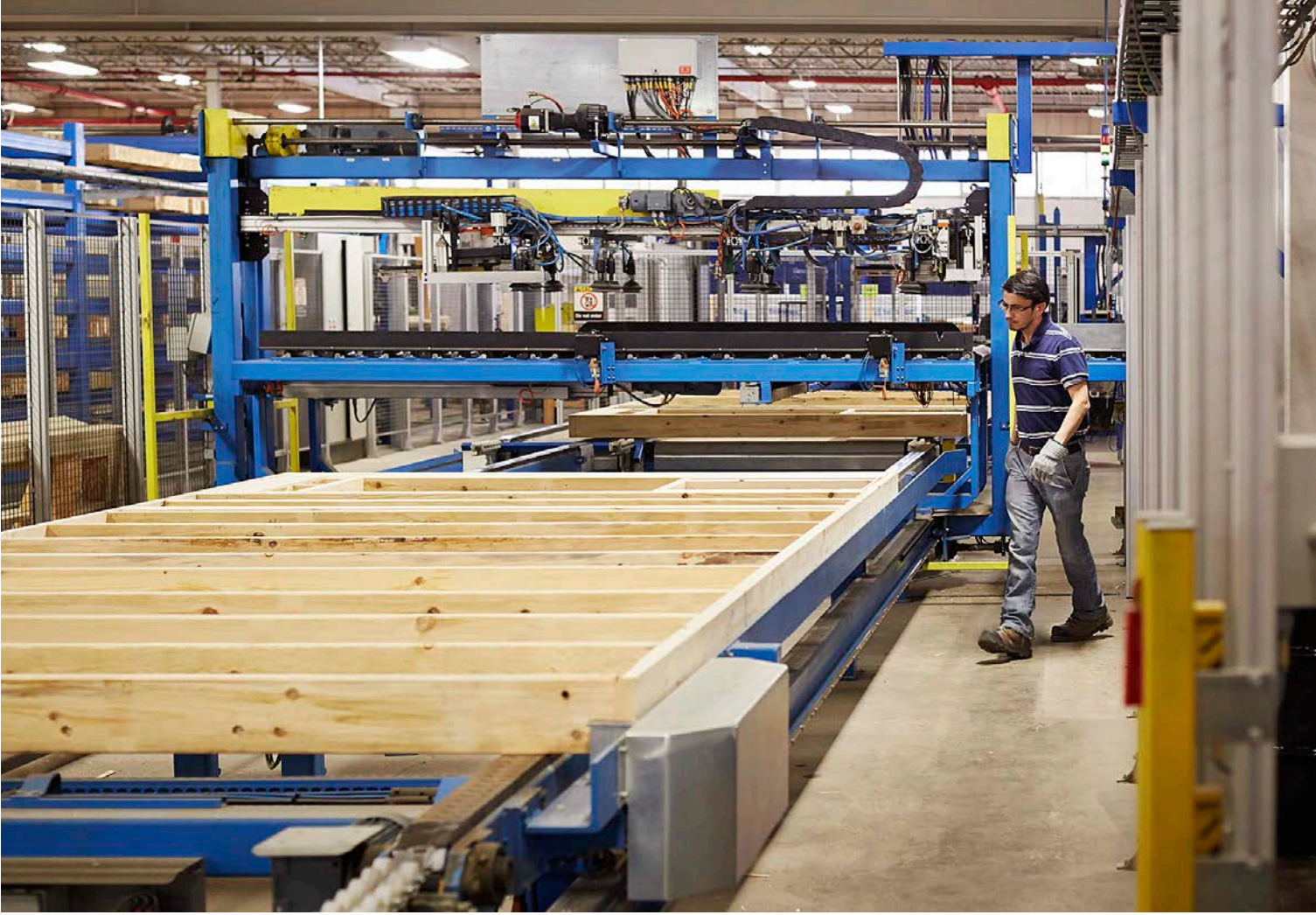
Brockport Homes’ pre-made panels are used for walls, floors and roofs that be can constructed in weeks rather than months.
