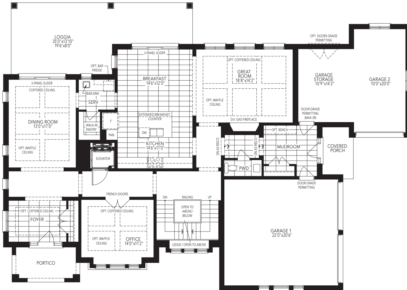
GROUND FLOOR W/OPT. ELEVATOR ELEVATION A
