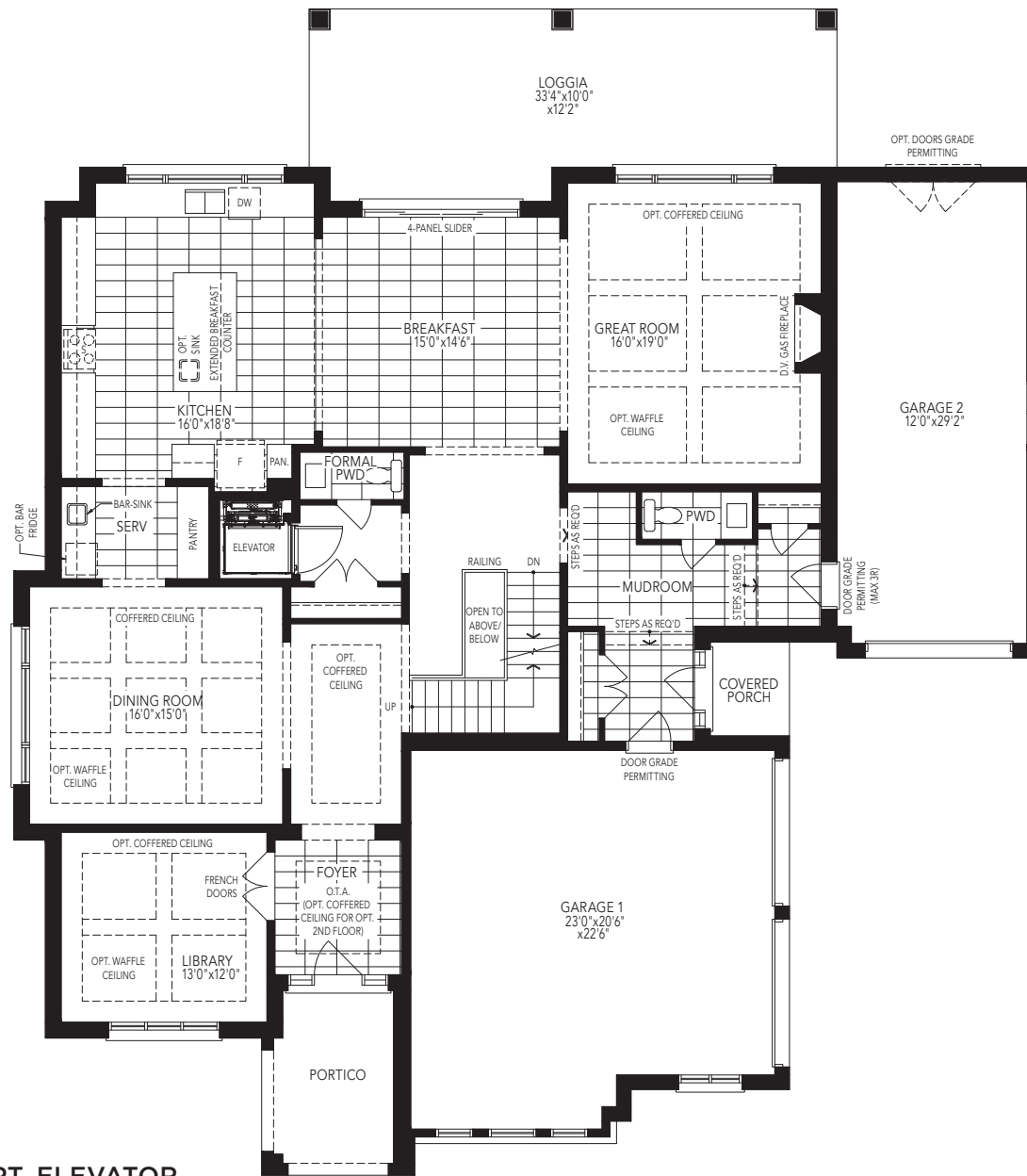
GROUND FLOOR W/OPT. ELEVATOR ELEVATION A
